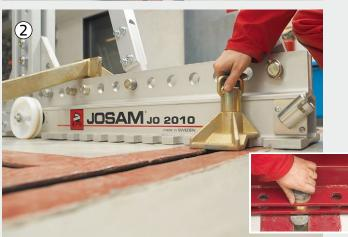
The I-beam anchoring fits in the same anchoring holders as the JOSAM frame straightening system. With a simple twist the cab tower is fastened into the I-beam in the workshop floor. Of course, our JOSAM cab bench also fits in the I-beams.
