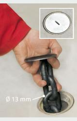
The floor anchoring is easy to install in your workshop floor in order to fix the cab tower, chains, anchoring beam or the JOSAM cab bench. The cab bench is fastened with four bolts (see left). When the "expander holes" are not in use they can simply be covered by a protective cover.
