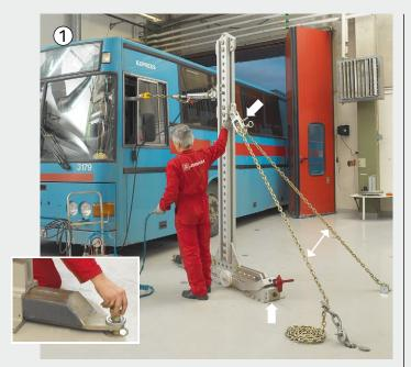
The floor anchoring is exceptional when it comes to repair of minor damage, as for this coach. In this case the cab tower is fixed with a nose bracket directly in the expander hole at the front and with chains at the rear. The tower is pretensioned with an impact wrench (see lower arrow). The pulling angle is quickly adjusted sideways and the tower locked into position with a pin (see upper arrows).
