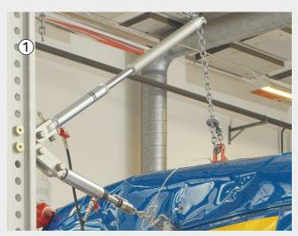
No matter which alternative is chosen, JOSAM cab tower can be utilized for many different repair jobs, thanks to its versatility. Here, for instance, a straightening job with advanced vector pulling is performed at 3-4 meters' height. In this case, our floor anchoring version is being used. Upwards vector pulling is only possible with this solution.
